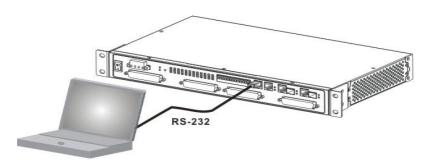
Figure 4-3 NCT480 Console Port Management Cabling
